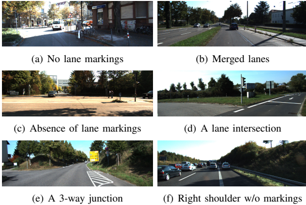
Fig. 6. Typical scenarios of abnormal lane markings. Figures labels correspond to those in Fig. 5.
