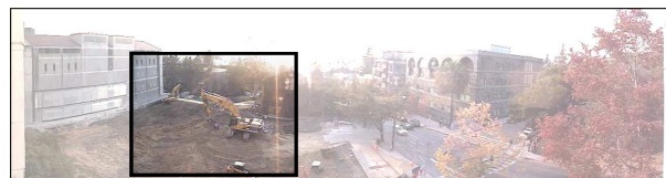
Fig. 1. Top Figure (a) illustrates system architecture; camera motion is determined by a combination of preset points, human inspector commands, and motion detector inputs. The resulting video sequences are aligned and inserted into the evolving panorama. Lower Figure (b) illustrates panoramic interface, the inset frame is a sample detail captured by the robotic camera and insertion algorithms.
