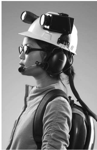
Figure 5.3: The human Tele-Actor transmits images from the remote environment using the helmet-mounted video camera and responds to user votes. Helmet design by E. Paulos, C. Myers, and M. Fogarty.
