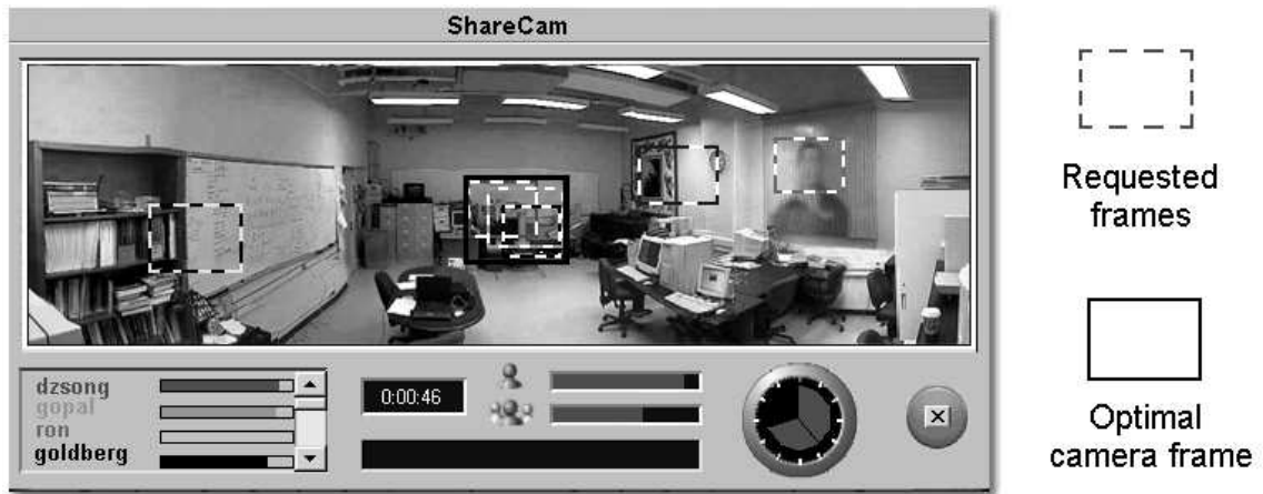
Figure 2.2: This figure illustrates the Co-Opticon's Java-based user interface, which currently runs on most Windows based PCs. Users view two windows. One (not shown) displays a live video stream as captured by the robotic camera. The second window, illustrated here, contains the user interface. The panoramic image is a fixed photo of the camera's reachable range of view. The snapshot above shows 6 active users listed in the scrollable window at the left. Each user requests a camera frame by positioning a dashed rectangle over the panoramic image. Based on these requests, the algorithm computes an optimal camera frame (shown with solid rectangle), and servoes the camera accordingly to displays the resulting live video stream. The horizontal bars indicate levels of user satisfaction as described below. The system is installed in our research lab at Berkeley and moved outdoors in June 2003. See: http://www.co-opticon.net
