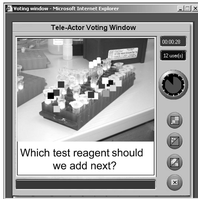
Figure 5.1: The Spatial Dynamic Voting (SDV) interface as viewed by each user. In the remote environment, the Tele-Actor takes images with a digital camera which are transmitted over the network and displayed to all participants with a relevant question. With a mouseclick, each user places a color-coded marker (a “votel” or voting element) on the image. Users view the position of all votels and can change their votel positions based on the group’s response. Votel positions are then processed to identify a “consensus region” in the voting image that is sent back to the Tele-Actor. In this manner, the group collaborates to guide the actions of the Tele-Actor.
